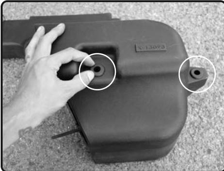
**13.** Install the remaining 2 grommets to the holes on bottom of injen air box and secure.
