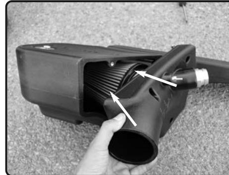
**3.** Install the plenum assembly into the air box.
