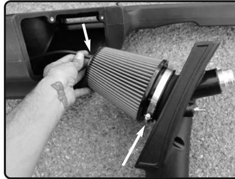
**14.** Install the filter to the plenum and tighten using 8mm nut driver. Connect the 3mm vacuum line from the filter minder to the barbed fitting on top of the filter.
