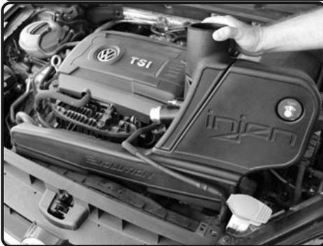
**5.** Install the intake assembly into the vehicle. Position to factory holes. Make sure the intake assembly seats in studs. *Note: Use lubrication to grommets for easier installation.*
