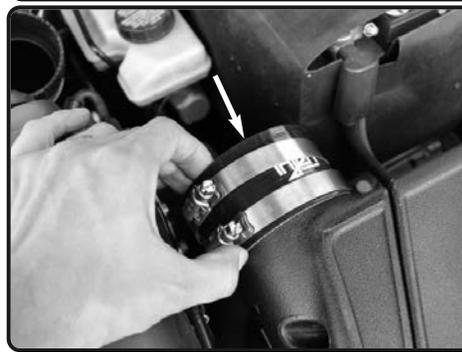
**7.** Install the 3.5" hump hose to the plenum. Do not Tighten.
