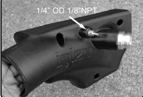
**9.** Install and secure the 1/8" NPT fitting to the plenum insert and tighten.
