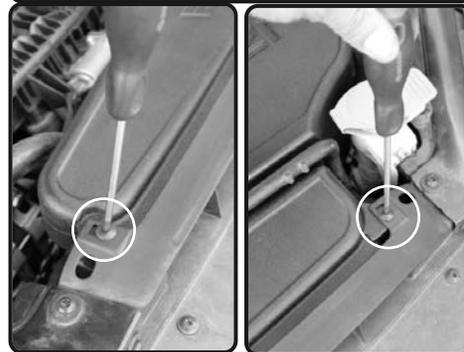
**6.** Now secure the injen Ram scoop using the factory screws from step 6.
