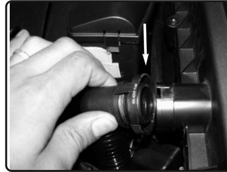
**3.** Pinch the harness on smog pump and pull away from air box. (if equipped with smog pump)
