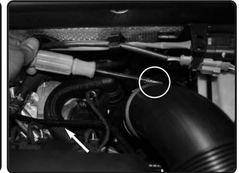
**4.** With 7mm nut driver, loosen the clamp on turbo housing.
