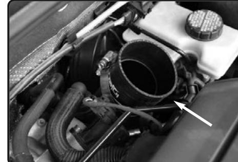
**10.** Install the 2-3/4"x3" step hose with clamps provided to the turbo housing.
