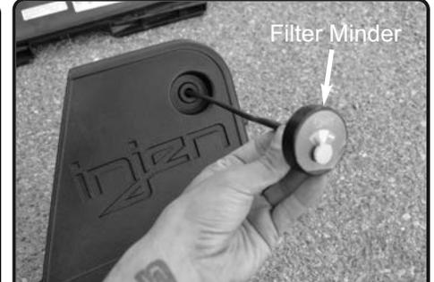
**12.** Attach the 3mm hose to the Filter minder and install the hose through the grommet.
