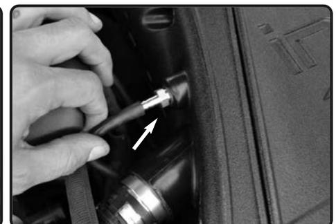
**12.** Now connect the vacuum line to the 1/4"OD NPT fitting.
