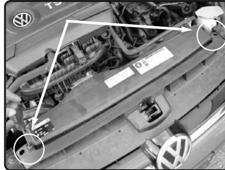
**6.** Loosen the 2 screws holding in the front OEM ram-scoop using T25 torx bit. Save screws for later install. Push clips down out of the radiator support.
