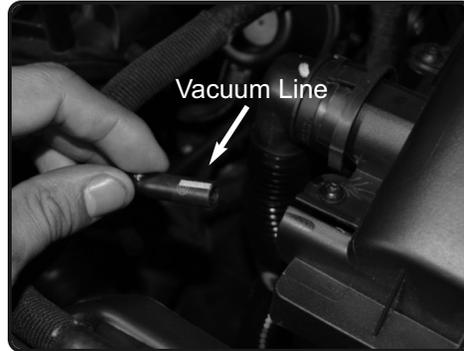
**2.** Remove small vacuum line from the factory airbox.
