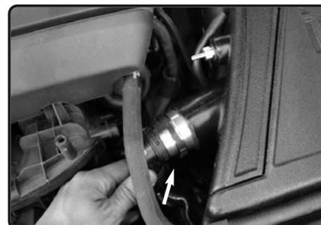
**11.** Connect the smog pump harness to machined fitting on intake tube and secure.
