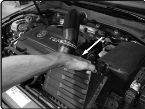
**5.** Now lift up OEM intake air box assembly out of vehicle.
