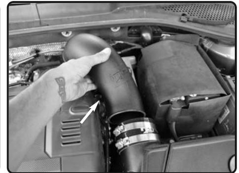
**8.** Install the intake tube to the vehicle. Position the tube to step hose and hump hose.
