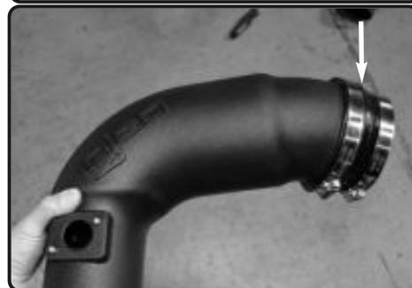
10. Place the 3.5"-4.0" step hose and one #64 and #56 clamps onto the turbo inlet side of the intake tube. Tighten the clamp on the turbo inlet side for now.
