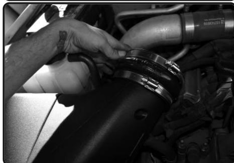
9. Place the 4.50" hump hose and two #72 clamps onto the Injen intake plenum. Secure the clamp on the plenum side for now.
