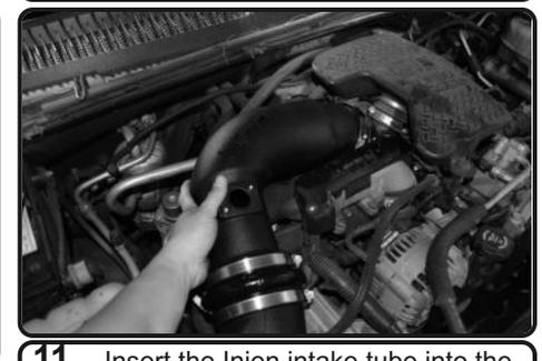
11. Insert the Injen intake tube into the 4.50" hump hose and the turbo end into the 3.5"-4.0" step hose. Once the intake is adjusted for best fitment, continue to secure the rest of the clamps
