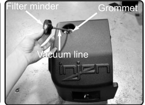
3. Place the grommet onto the drilled hole on top of the Injen air box. Connect the vacuum line to the filter minder then run the Filter minder into the grommet.
