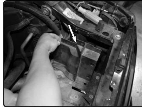
7. Remove the trim panel behind the passenger side headlight. Removing this panel will allow additional air into the intake system.
