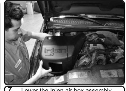
7. Lower the Injen air box assembly into the engine bay. Make sure the pegs under the injen air box goes into the factory air box grommets located on the air box bracket.
