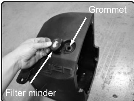
5. Place the grommet onto the drilled hole on top of the Injen air box. Push the Filter minder into the grommet.
