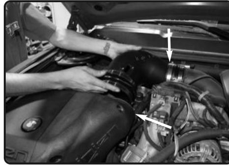
**14.** Place the small end of the Injen tube into the 4.125" straight hose on the turbo inlet and the other end into the Injen air box. Slide the 5.00" hump hose over the Injen air box
