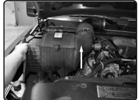
4. Firmly lift up on the stock air box assembly and pull the stock air box assembly out of the engine bay.
