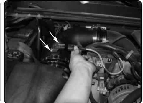
**16.** Place the MAF sensor into the Injen tube. Secure the MAF sensor to the tube with two M4 button head bolts. Re-connect the MAF sensor harness
