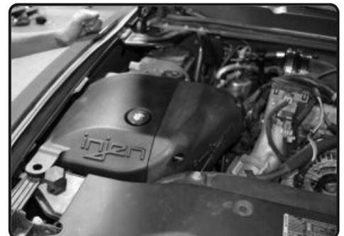
12. Drop the Injen air box onto the grommets from figure 11. Make sure the two mounting nipples underneath the Injen air box goes directly into the grommets.
