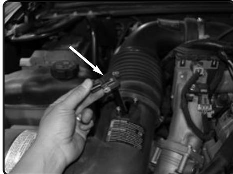
2. Disconnect the MAF sensor harness. Loosen two torx bits and remove MAF sensor from the stock air box assembly.
