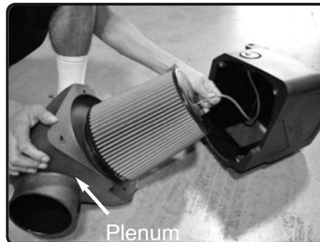
7. Place the filter onto the plenum and secure the clamp. Then connect the 3mm vacuum hose from figure 6 to the barbed fitting on the filter
