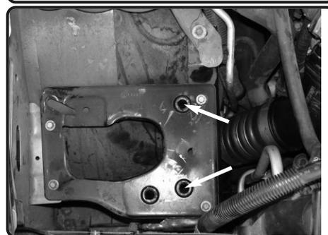
11. The factory air box assembly bracket is shown in the photo. Arrows indicate the grommets where the Injen air box mounts will go
