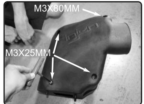
8. Place the three M6X25mm bolts and one M6X80mm into the plenum illustrated by the photo
