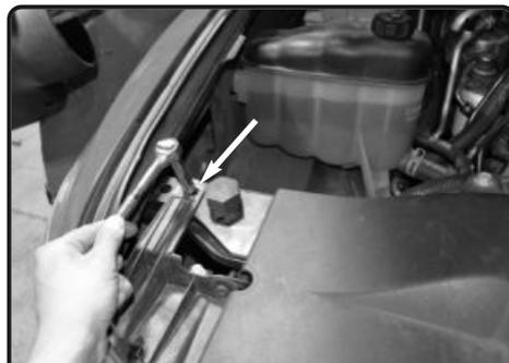
10. Use a 10mm socket/ratchet to remove the 10mm bolt from the passenger-side headlight.
