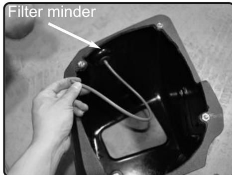
6. Connect the 16"- 3mm vacuum line to the filter minder
