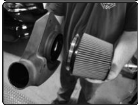
11. Place the filter onto the 6.00" opening on the intake plenum and then secure the clamp.
