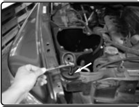
9. Once the Injen air box is mounted, use the factory 10mm bolt to secure the air box bracket to the radiator support.
