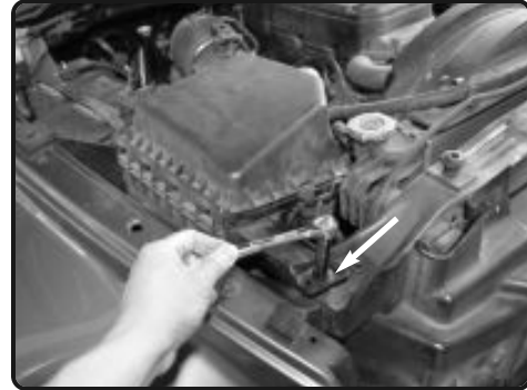
2. Use a 10mm socket/ratchet and remove the 10mm nut securing the stock air box assembly to the radiator support.
