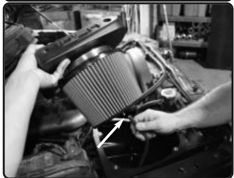
12. Connect the 3mm vacuum hose from figure 10 to the Filter Minder to the barbed fitting on top of the Injen filter.
