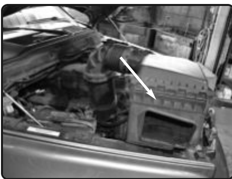
5. Pull the air duct off the turbocharger and then firmly lift up on the entire air box assembly and remove the entire stock air box assembly from the engine bay
