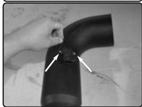
7. Place the AIT sensor into the Injen intake tube and two M4X16 bolts to secure it to the tube with an allen key.
