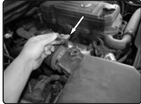
3. Disconnect the AIT sensor harness and then remove the two 7mm screws to remove the AIT sensor from the stock air box assembly
