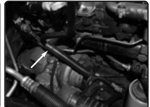
**8.** Connect the 17"-7mm vacuum hose to the crank case breather line. This vacuum line will connect to the Injen intake tube in figure 16
