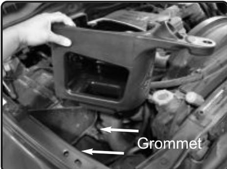
**9.** Drop the Injen intake box into the OE air box location. Line up the two mounting taps underneath the Injen air box to the two factory mounting grommets.
