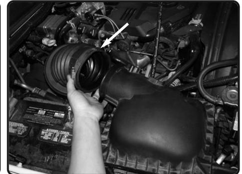
**4.** Loosen the clamp from the air duct to the air box assembly and then pull the air duct from the air box.
