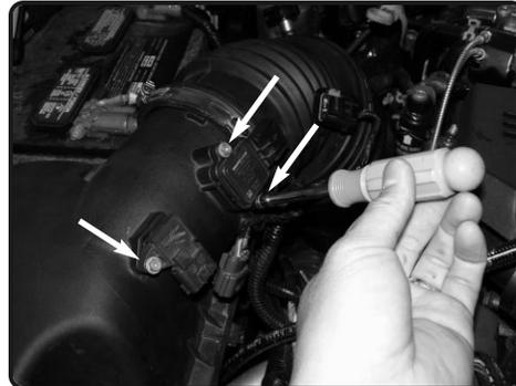
**2.** Disconnect the MAF/AIT sensor harness and then use a 7mm nut driver to loosen 3-7mm screws from the sensors. Remove sensors from the air box for now
