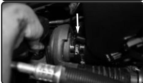
**17.** Once the intake tube is lined up with the turbocharger inlet, slide the 4.00" straight hose from figure 14 over the turbo inlet. Also connect the vacuum line to the CCV line to the Injen intake tube from figure 8
