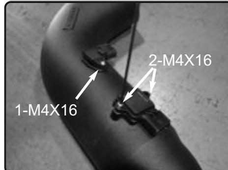
**7.** Place the MAF/AIT sensor into the Injen intake tube. The two M4X10 bolts are for the MAF sensor and the one M4X16 bolt is for the AIT sensor.
