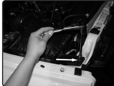
**3.** Remove the 10mm nut from the air box assembly on the radiator support.
