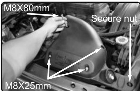
**13.** Place the three M8X25mm bolts and one M8X80mm bolt to the top of the plenum illustrated by the photo and then secure the bolts with a philips. Use the factor 10mm nut to secure the air box bracket to the radiator support.
