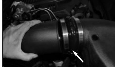
**18.** Push the upper part of the intake tube into the 4.50" hump hose on the intake plenum. Slide the hump hose towards the intake tube till it's centered. Adjust intake tube for best fitment and then secure all the clamps.
