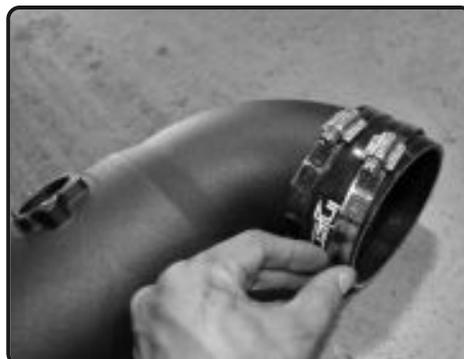
**15.** Place the 4.00" straight hose and two #64 clamps onto the small end of the intake tube. Make sure you slide the straight hose as far back as you can.
