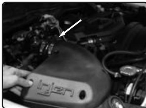
**14.** Place the 4.50" hump hose and two #72 clamps onto the intake plenum. Make sure you slide the hump hose as far back as you can.
