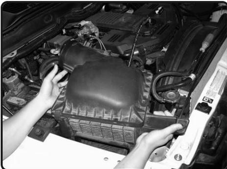
**5.** Firmly lift up on the entire air box assembly and remove it from the engine bay.
