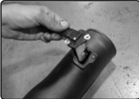
**13.** Remove the MAF sensor from the factory airbox assembly and put the MAF sensor into the new Injen intake tube. Use two M4 bolt and secure the MAF sensor to the Injen tube with an allen key
