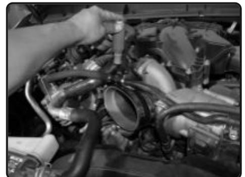
12. Place the 4.50" straight hose and two #72 clamps onto the turbo inlet. Only secure the clamp on the turbo inlet for now.
