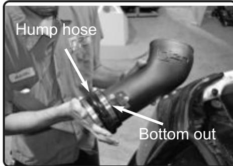
**14.** Place the 4.50" hump hose and two #72 clamps onto the round end of the Injen intake tube. Make sure you push the hump hose all the way down to the MAF sensor
