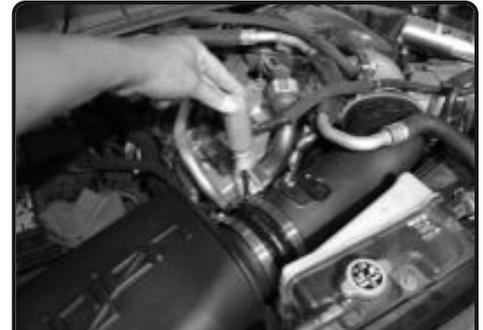
**16.** Connect the other end of the tube to the Injen air box plenum and push the 4.50" hump hose over. Adjust the intake system for best fitment and secure clamps.
