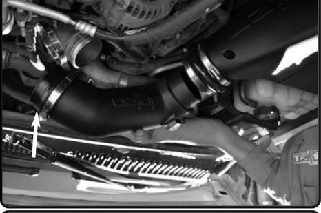
**12.** Place the 3.5"-4.0" step hose and one #64 and #56 clamps onto the turbo inlet side of the intake tube. Tighten the clamp on the turbo inlet side for now.
