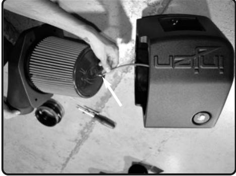
**5.** Connect the 3mm vacuum hose from figure 6 to the barbed fitting on the filter
