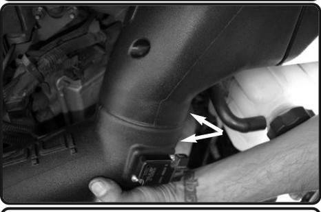
**10.** For illustrative purposes only: Step down section of the Injen intake tube shown fully bottomed out into the Injen intake plenum. Proceed to the next step to install the required hump hose.
