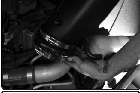
**11.** Place the 4.50" hump hose and two #72 clamps onto the Injen intake plenum. Secure the clamp on the plenum side for now.
