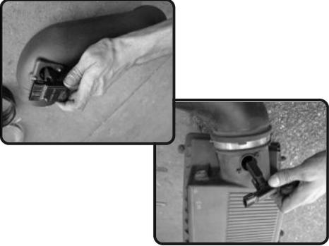
**8.** Remove the factory MAF sensor from the factory air box assembly and then install it into the Injen intake tube. Use two M4 supplied bolts to secure it to the tube.
