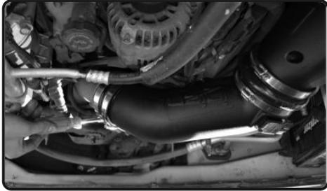
**13.** Insert the step down section into the intake plenum. Make sure the step down section bottoms all the way into the intake plenum (refer to figure 9&10). Insert the other end into the turbo inlet. Adjust the intake system for best fitment and then continue to secure the rest of the clamps
