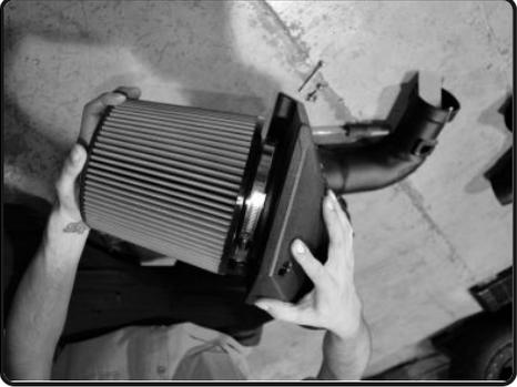
**4.** Place the filter onto the the Injen intake plenum and then secure the clamp.
