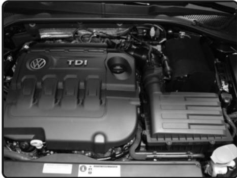
**1.** Stock box shown in this picture, if desired remove the engine cover for easier installation.
