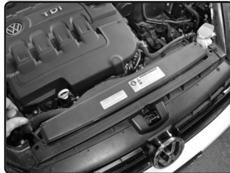
**6.** With T25 torx bit, loosen the 2 bolts holding in the OEM ram-scoop. Save bolts for later install.
