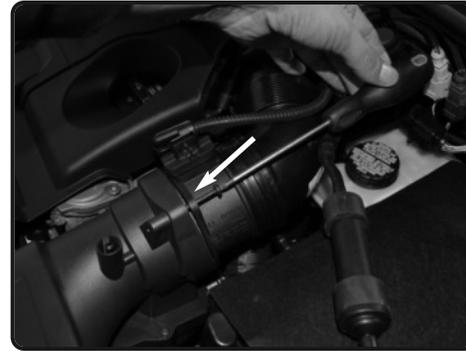
**3.** With T25 torx bit, loosen the 1 screw holding in MAF sensor.
