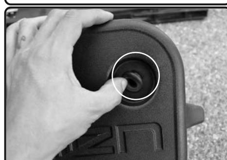
**11.** Install the provided grommet to the filter minder hole cut-out on Injen air box.
