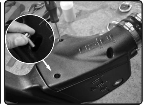
**4.** Secure using the 3 provided M6x20mm phillips screw with rubberized washer.
