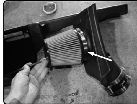
**3.** Connect the 3mm vacuum line from the filter minder to the barbed fitting on top of the filter. Install the plenum assembly into the air box.
