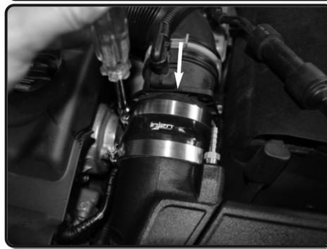
**7.** Install the MAF sensor into the step hose. Secure the MAF sensor clamp using 8mm nut driver.
