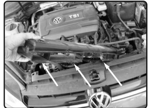
**8.** Now carefully pull back, and pull out the OEM ram-scoop from vehicle.
