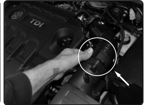
**4.** Rotate the MAF sensor towards the battery. This will unlock the bottom of the MAF sensor.
