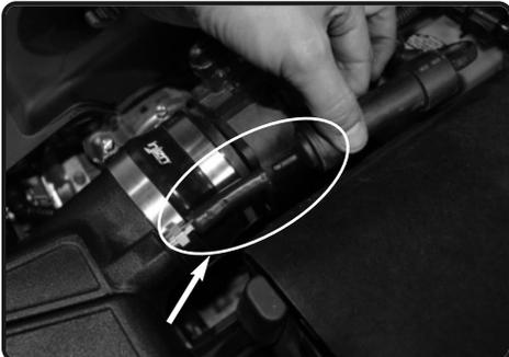
**9.** Now connect the vacuum line to the hose and secure.
