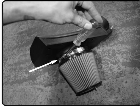
**14.** Install the filter to the plenum and tighten using 8mm nut driver.
