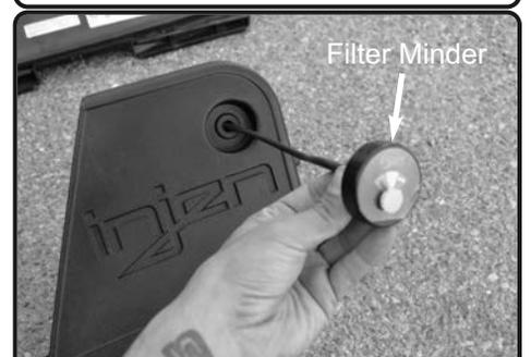
**12.** Attach the 3mm hose to the Filter minder and install the hose through the grommet.
