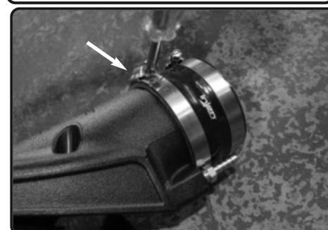
**10.** Install the step hose with clamps provided to the plenum. Tighten the clamp on the plenum using 8mm nut driver.
