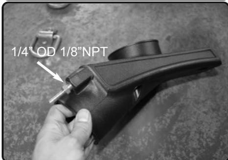
**9.** Install and secure the 1/4" NPT fitting to the plenum insert and tighten using 1/2" wrench.
