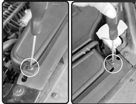
**6.** Now secure the injen Ram scoop using the factory screws from step 6.
