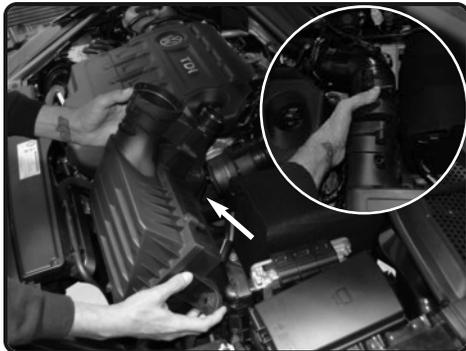
**5.** Now carefully pull back the MAF sensor from the airbox. Lift up and remove the air box box from vehicle.
