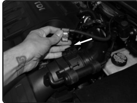
**2.** Disconnect MAF sensor harness. Disconnect and remove the small vacuum line.
