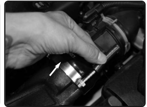
**8.** Install the provided the 4mm hose to the fitting.
