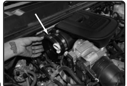
12. Place the 4.25"-4.50" step hose and two #72 clamps onto the turbo inlet. Tighten the clamp on the turbo inlet side for now.
