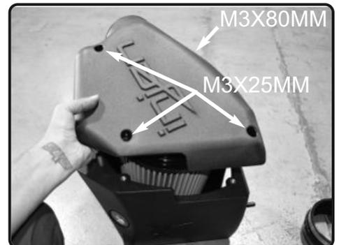
8. Place the three M6X25mm bolts and one M6X80mm into the plenum illustrated by the photo. Your Injen air box assembly is now complete.
