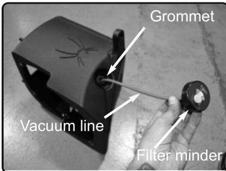
5. Place the grommet onto the drilled hole on top of the Injen air box. Connect the vacuum line to the filter minder then run the Filter minder into the grommet.
