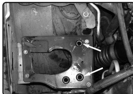
10. The factory air box assembly shown in the photo. Arrows indicate the grommets where the Injen air box mounts will go.
