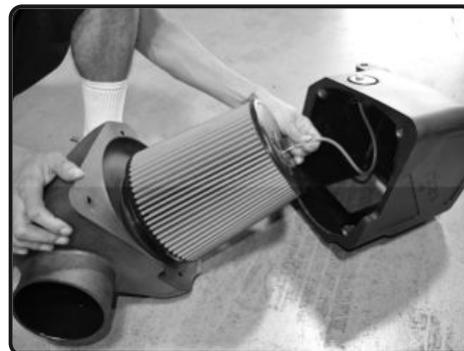
7. Connect the 3mm vacuum hose from figure 6 to the barbed fitting on the filter
