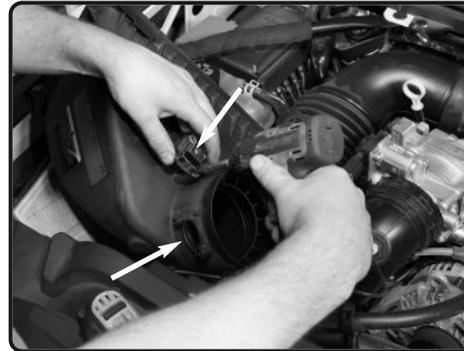
3. Remove the factory the two maf sensors from the factory air box assembly.
