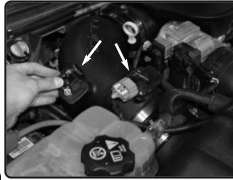
**15.** Place both MAF sensors onto their appropriate location and then screw them down with the supplied M4 bolts. Reconnect the MAF sensor harnesses
