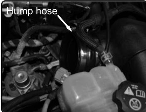
**13.** Place the 5.00" hump hose and two #80 clamps onto the Injen intake plenum on the injen air box.
