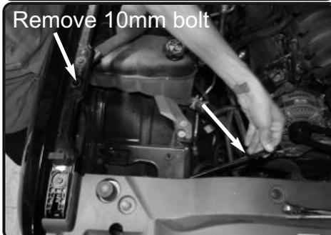
9. Remove the 10mm bolt from the support bracket and then swing the support bracket towards the right. This will allow you to install the Injen air box.
