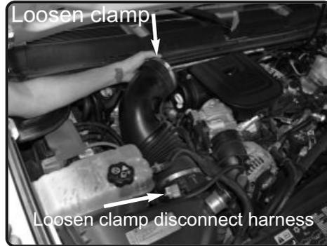
2. Disconnect the MAF sensor harness. Loosen the clamp on the intake duct and then remove entire air duct
