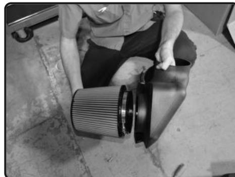
6. Place the filter onto the the Injen intake plenum and then secure the clamp.
