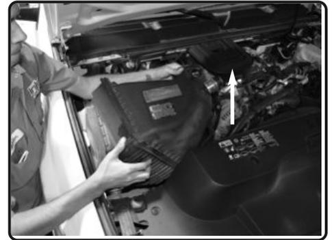
4. Firmly lift up on the stock air box assembly and pull the stock air box assembly out of the engine bay.
