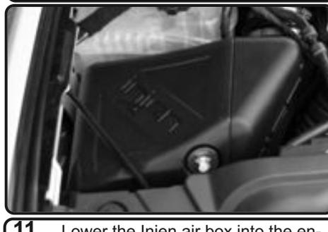
11. Lower the Injen air box into the engine bay. Make sure the pegs under the Injen air box goes into the factory air box grommets on the air box tray from figure 10. Also re-install the support bracket.
